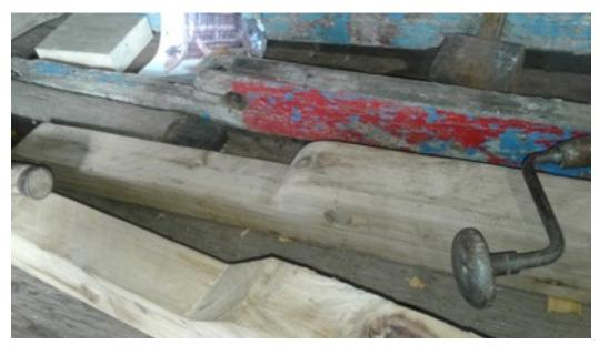
In the centre you can see the old part with the paint, and the new wider one just about completed. Of Course the old dray was built to Imperial measure (feet and inches) and the metric timber had to be cut down to original dimensions to fit the old metal parts, and be faithful to the original.
