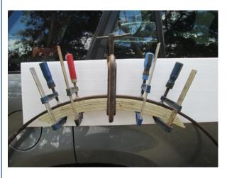
Now the tyre. Ordinarily with a new wheel the tyre would have been heated and shrunk on, but I had existing bolt holes in the tyre and rim and a cold fit to do if possible. One half was easy enough, the second rather awkward and I wasn't at all confident. However a collection of clamps of various sizes, a rubber mallet, some blood and skin, help from my Chinese grandma and a few judicious words and snap, it clicked into place just as a young Belgian couple strolled by.
